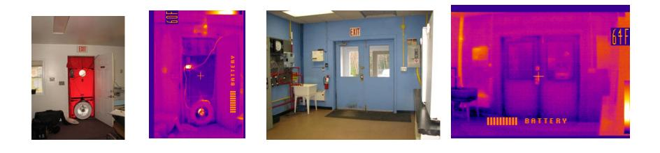
Garage door most significant contributor to air leakage. As they do not use this for vehicle storage, removing the door and framing in a 2x6 wall with one large oversized insulated door is recommended.
