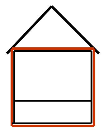
Heating equipment is supposed to be sized to be able to replace all the heat lost thorough the envelope in one hour during one of the coldest winter temps. The more effective the envelope performs, the less heat is lost – the less heat input is needed and the smaller the equipment!!!! (Or summer A/C units!)
