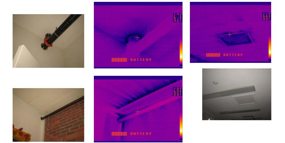
Attic's cellulose insulation ranges from 2-5" in depth in between joists for effective levels ranging from R6 to R15 with all framing approx R6. Residential codes call for R49 in New Hampshire. While non residential have lower requirements, low energy buildings often shoot for R50-R60!
