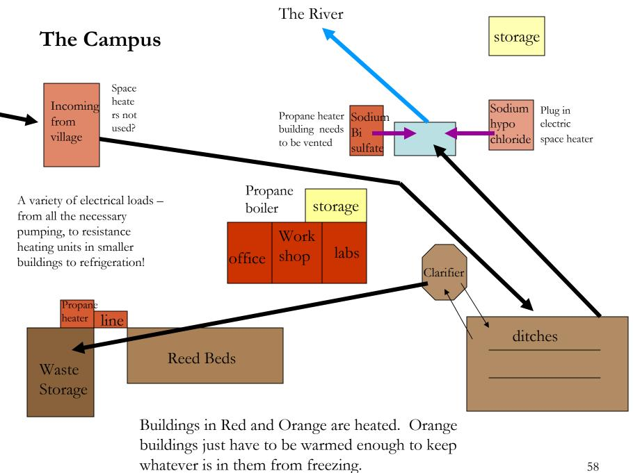
According to the records provided, this "Sludge Building" uses 1000 gallons a year to keep a pipe to the reed beds from freezing.
