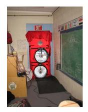
This means that at -50 pas (as if a 20mph wind was blowing on all sides of the building at once) the air would completely change **almost 6 times every hour**. The math: CFM50 x 60 / building volume Standard Residential Construction practices is generally between 7 and 9ACH50 and 2009 IECC sets 7ACH50 limit. Energy Star's limit is 5ACH50. High Performance Homes under 1ACH50. Currently no standard for non residential buildings.
