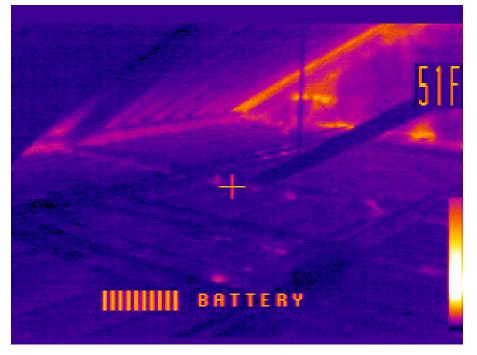
Ice dams form when roof sheathing is warmed from below. Heat loss above the top plate and warm air rising between framing members or other penetrations are often likely suspects.
