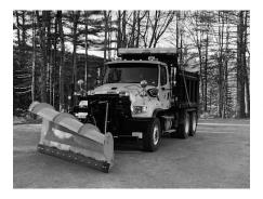
We took delivery of the new 2021 Freightliner 10-wheeler that was ordered back in the fall of 2020. This unit will replace the 1997 Mack dump truck. The new truck is equipped with a combo dump body/sand salt spreader.
